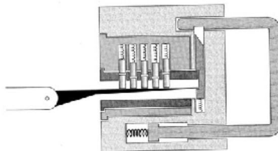
Figure 11. Bypass picking <sup>39</sup>
