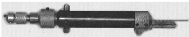
Figure 9. A pin lock decoder tool for measuring the bottom pins of a lock<sup>35</sup>
