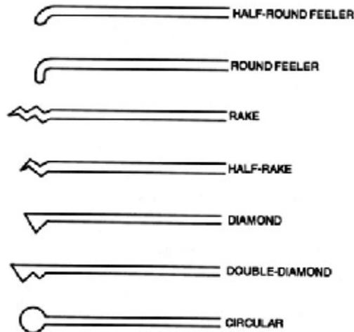
Figure 4. Some basic lockpick shapes<sup>18</sup>
