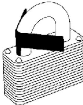
Figure 10. Opening a padlock with a shim <sup>37</sup>
