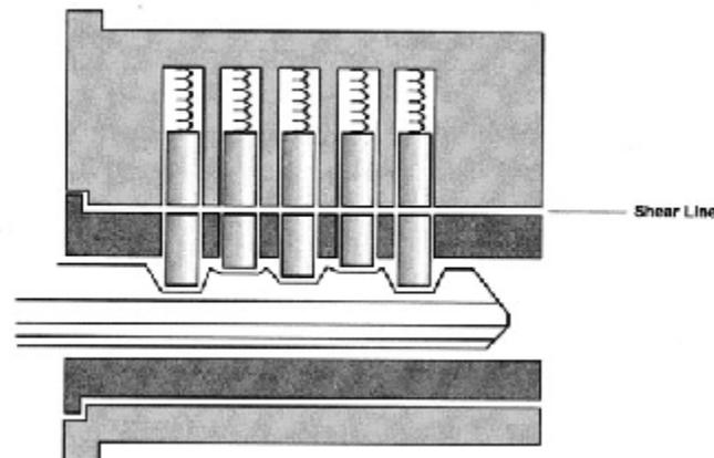
Figure 2. Side view cutaway – key inserted<sup>10</sup>
