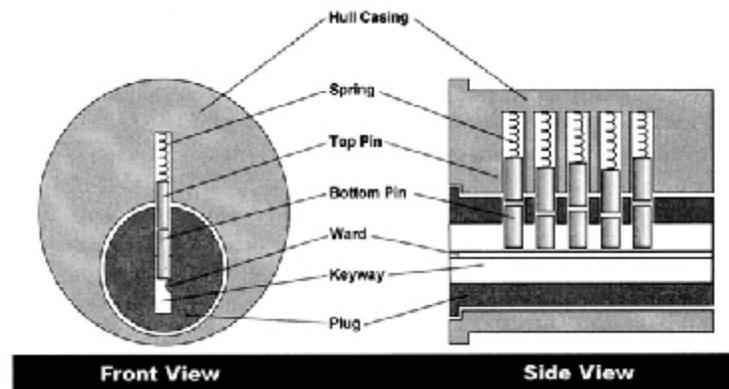
Figure 1. Parts of a Pin Tumbler lock<sup>9</sup>
