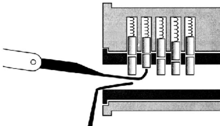
Figure 5. Placement of Pick and Tension Wrench in the lock keyway for picking <sup>20</sup>
